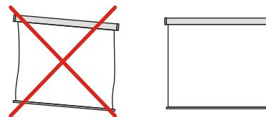
In order to get a stable position of the screen, it is important to hang up the casing exactly horizontally.
